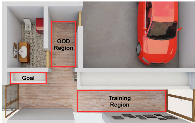
Fig. 11: Unvisited Area OOD setup. During evaluation, one sandal and one shoe from the four target objects are placed in a region where no target objects appear in the training demonstrations.
